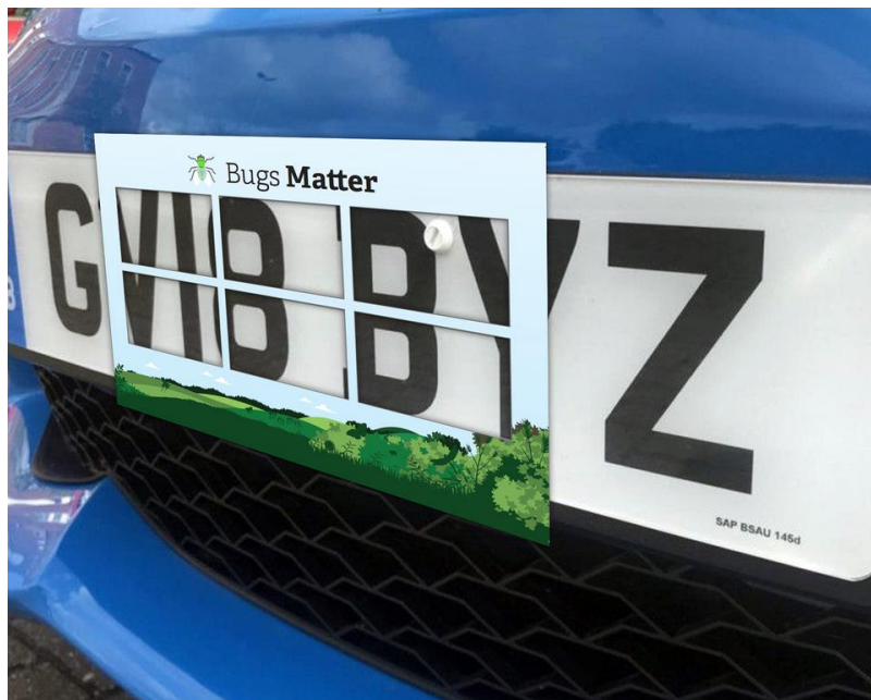
Figure 2. Photograph showing the splatometer positioned over a number plate.
